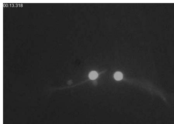
FIGURE 5 Fluorescence image shows the broken MT under external force on it.
